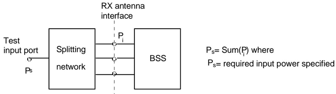
**Figure B.1: Receiver test set-up**
