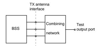
Figure B.2: Transmitter test set-up
