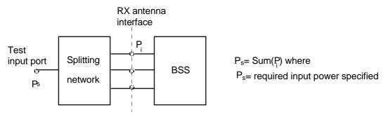
Figure B.1: Receiver test set-up
