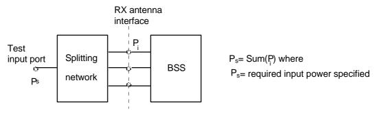
Figure B.1: Receiver test set-up
