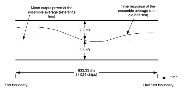
Figure 2: Transmission envelope mask (average non-idle half slot)
