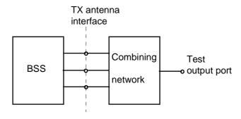
Figure B.2: Transmitter test set-up
