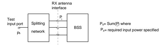
Figure B.1: Receiver test set-up
