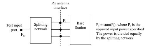
Figure B.5.1-1: Receiver test set-up
