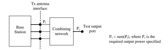
Figure B.5.2-1: Transmitter test set-up
