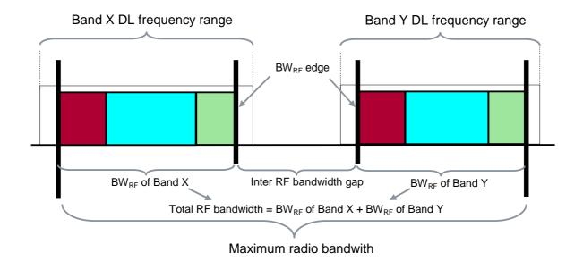
Figure 3.2-1: Illustration of Maximum Radio Bandwidth BW<sub>max</sub> and Total RF Bandwidth for Multi-band Base Station BW<sub>tot</sub>
