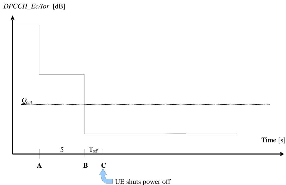
**Figure 4.2.11.2-1: Conditions for out-of-synchronization handling in the UE****Table 4.2.11.2-2: Conditions for out-of-synchronization handling in the UE**
