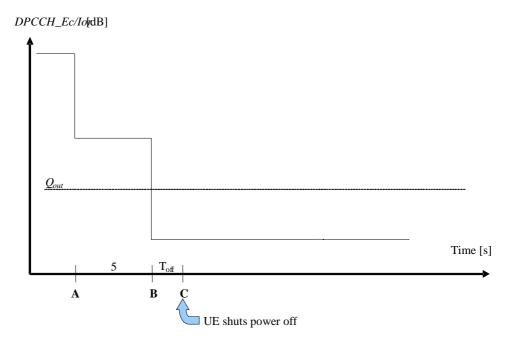
Figure 4.2.11.2-1: Conditions for out-of-synchronization handling in the UE
