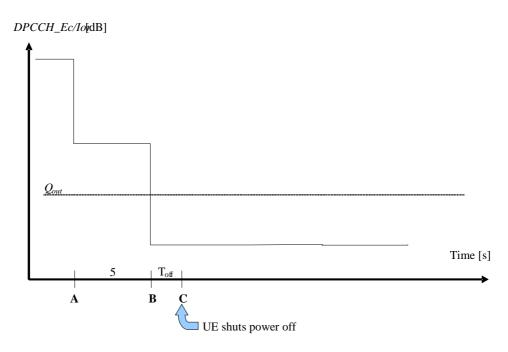
Figure 4.2.11.2-1: Conditions for out-of-synchronization handling in the UE
