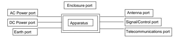
Figure 2: Examples of ports
