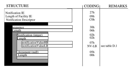
Figure D.6: Encoding of call intrusion notifications
