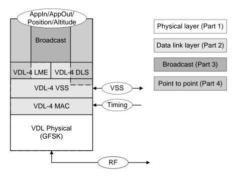
Figure 4.2: Structure of VDL Mode 4 ground station specifications
