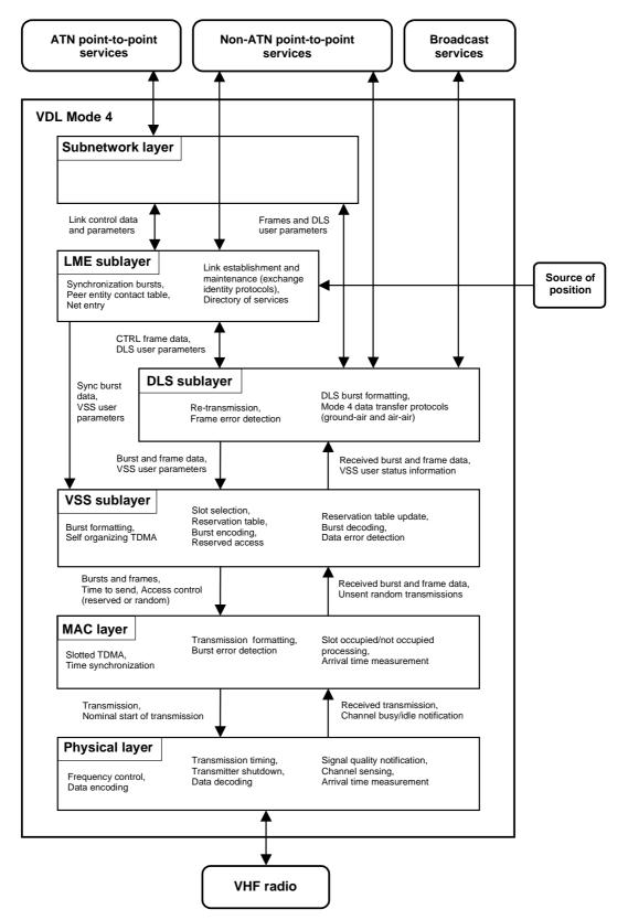
Figure 4.1: Layered structure of VDL Mode 4
