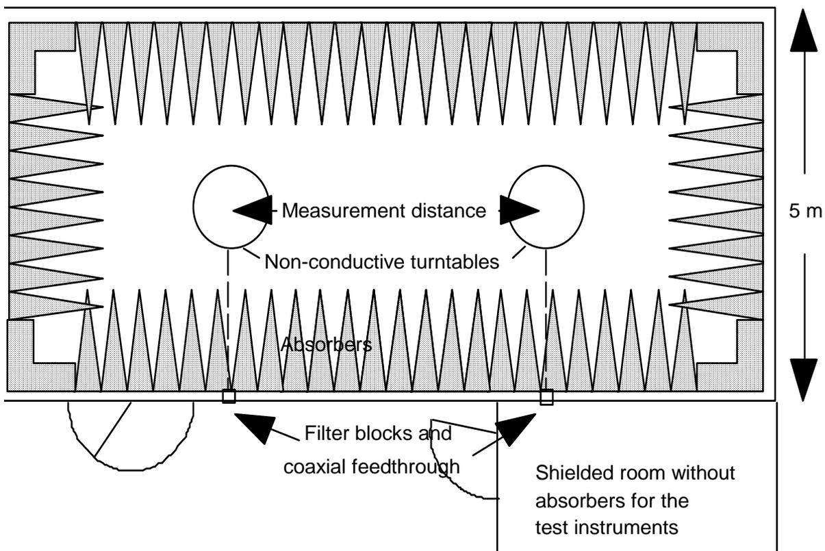
Figure A.5: Example of construction of an anechoic shielded chamber
