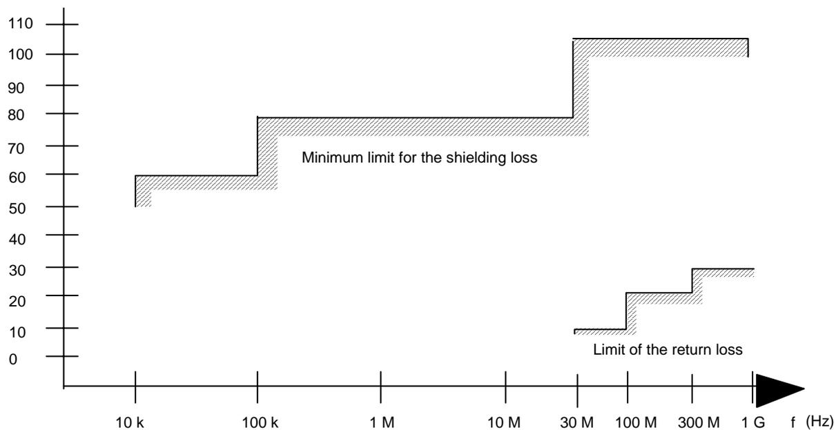
Figure A.4: Specification for shielding and reflections
