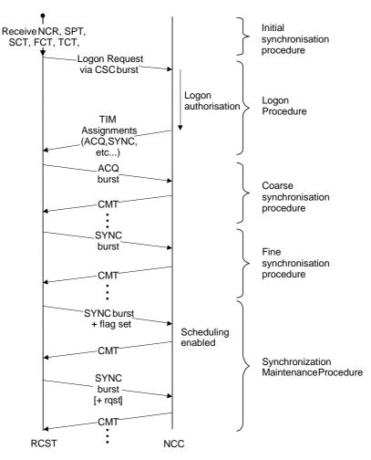
Figure 26: Example of RCST network entry signalling flow
