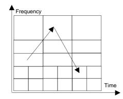
Figure 21: Optional dynamic-Slot MF-TDMA, using a flexible RCST
