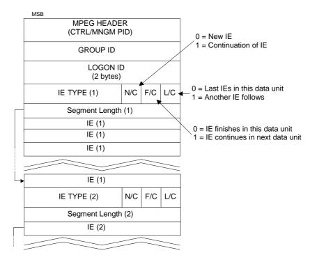
Figure 19: DULM over optional MPEG packets
