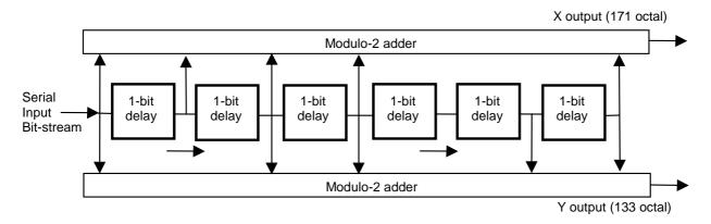
Figure 12: Convolutional code of rate 1/2
