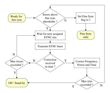
Figure 29: Fine synchronization procedure (optional)
