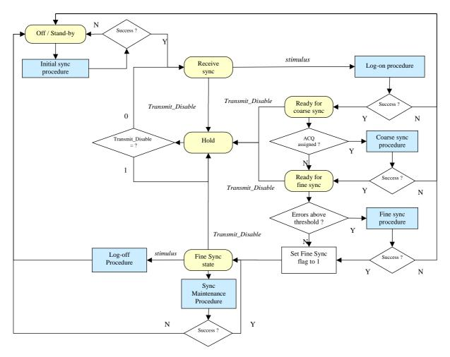
Figure 25: RCST synchronization state diagram
