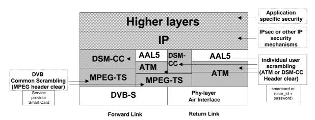
Figure 36: Security layers for satellite interactive network (example)
