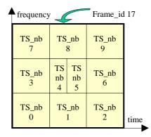
Figure 24: example of frame composition
