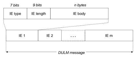
Figure 18: DULM message with ATM TRF bursts
