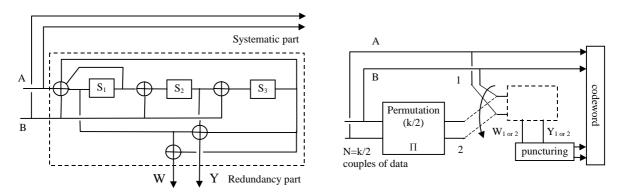
Figure 13: Encoder block diagram (turbo code)
