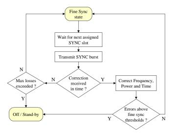
Figure 30: Synchronization maintenance procedure
