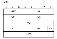
Figure 31: ATM cell header format
