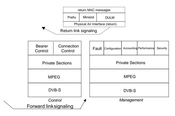
Figure 33: Protocol stack for signalling
