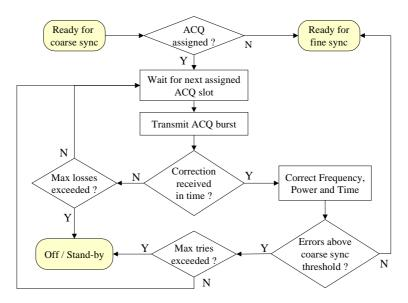
Figure 28: Coarse synchronization procedure (optional)
