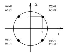
Figure 16: Bit mapping into QPSK constellation
