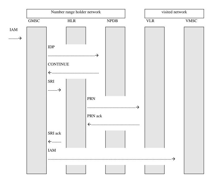
Figure A.2.4 shows the information flow for unsuccessful TQoD (number not ported).
