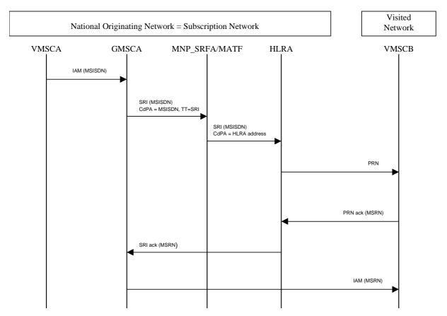
Figure C.4.2: Successful delivery of a call to a ported number via direct routeing where the call is originated in the subscription network
