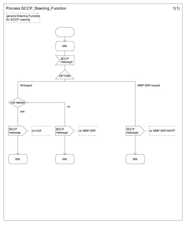
Figure 1: Steering Function for SCCP Message routeing
