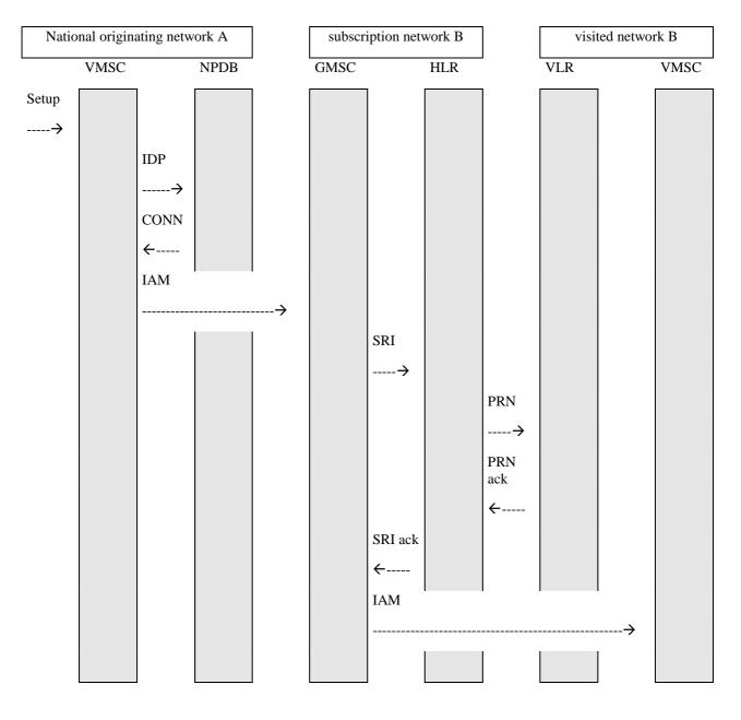
Figure A.2.5 shows the information flow for successful OQoD (number ported).
