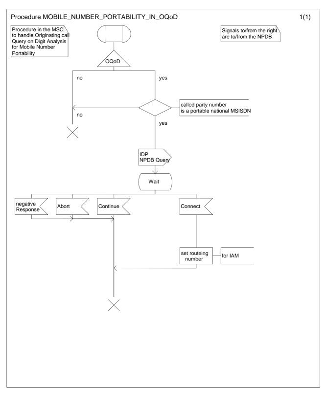
Figure A.3.3: Procedure MOBILE\_NUMBER\_PORTABILITY\_IN\_OQoD
