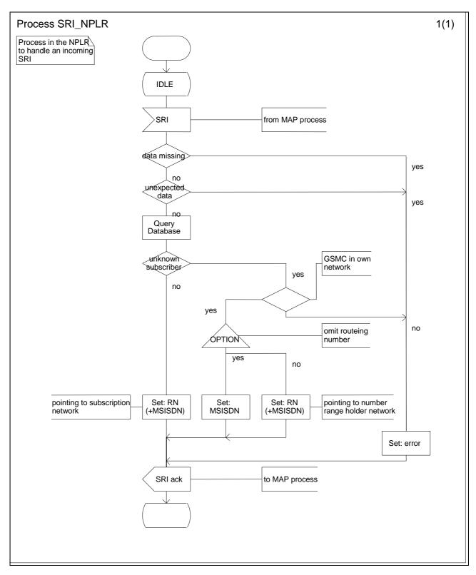
Figure C.2.2: Process SRI\_NPLR
