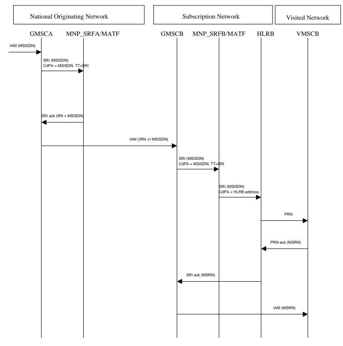
Figure C.4.3: Successful delivery of a national mobile originated call to a ported number via direct routeing
