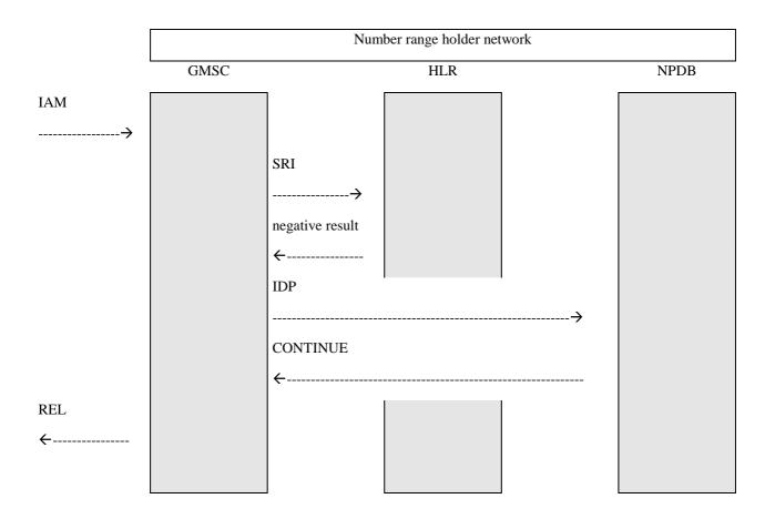
Figure A.2.2 shows the information flow for unsuccessful QoHR (misdialled unallocated number).
