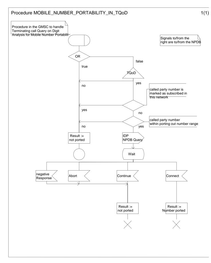
Figure A.3.2: Procedure MOBILE\_NUMBER\_PORTABILITY\_IN\_TQoD
