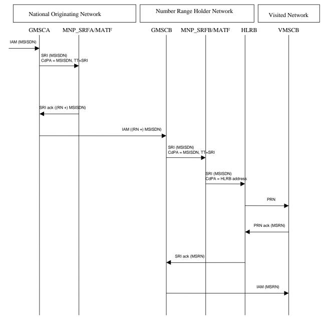
Figure C.4.4: Successful delivery of a national mobile originated call to a not known to be ported number via direct routeing
