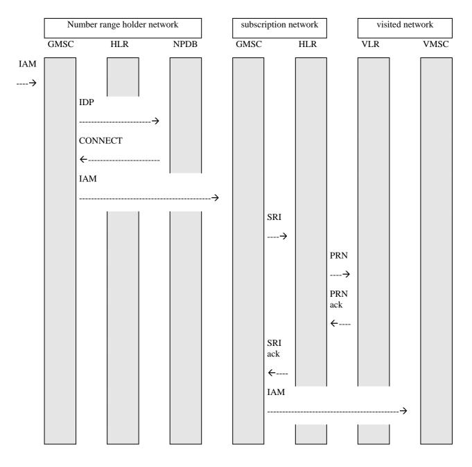
Figure A.2.3 shows the information flow for successful TQoD.
