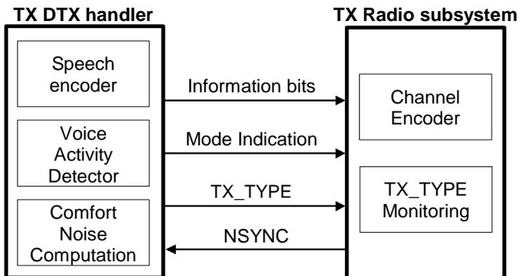
Figure 1: Block diagram of the transmit side DTX functions
