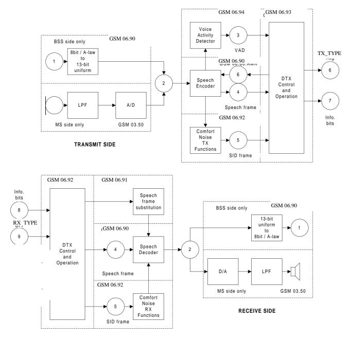
Figure 1: Overview of audio processing functions
