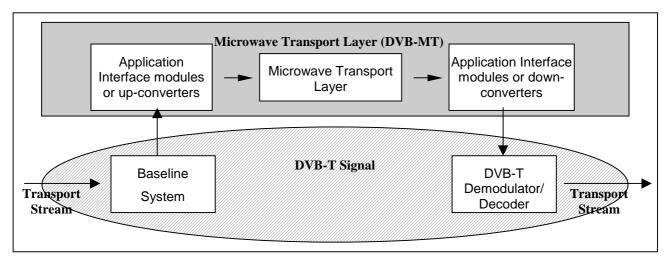
Figure 2: Functional block diagram of the Baseline & Transport System
