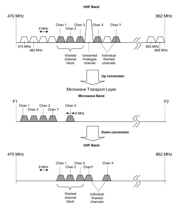
Figure 3: Example of frequency translations between UHF and Microwave for an 'off air' fed system
