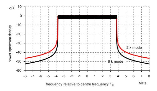
Figure 4: Theoretical UHF DVB transmission signal spectrum for guard interval  $\Delta = T_u/4$
