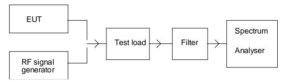
Figure 6: Measurement arrangement for conducted emissions
