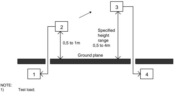
MES under test (antenna port connected to the test load); 2)
