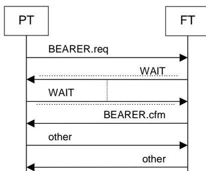
Figure 8: PT initiated setup of initial duplex bearer
