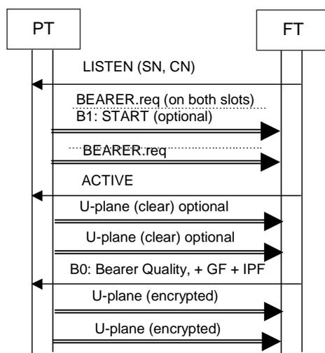
Figure 11: Successful upstream direct double simplex bearer setup
