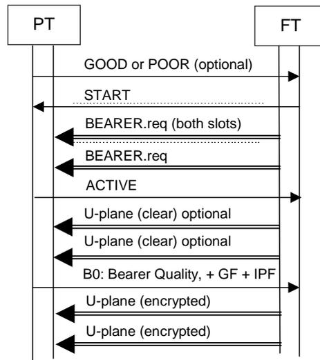
**Figure 12: Successful downstream direct double simplex bearer setup**
