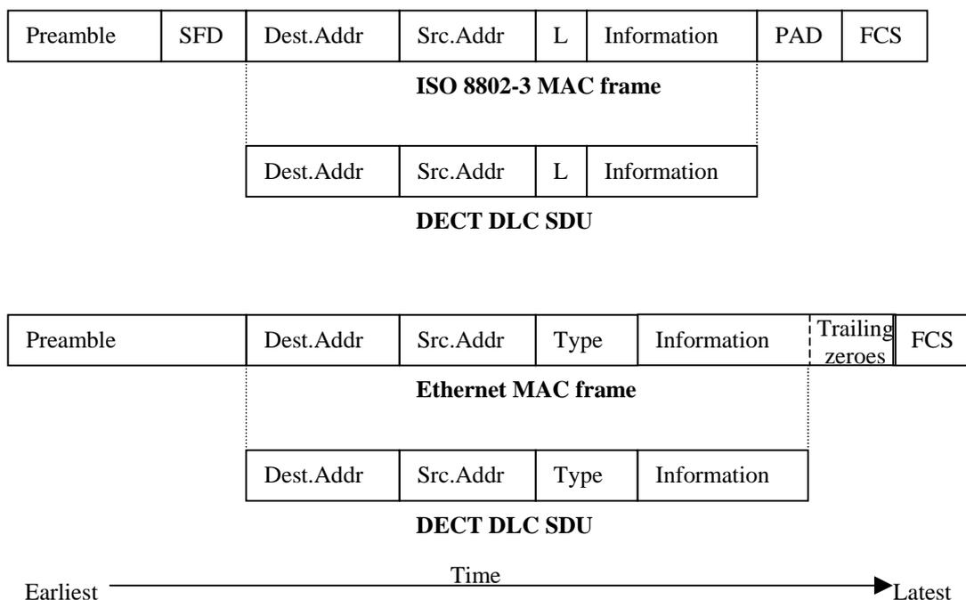
**Figure B.5: Mapping of IEEE 802.3 [13] and Ethernet MAC frames into DECT DLC SDU**
