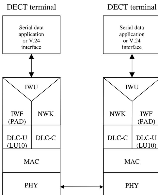
**Figure C.1: Reference configuration showing the DPRS V.24**
