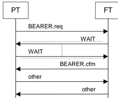
**Figure 10: PT initiated setup of additional duplex bearer**
