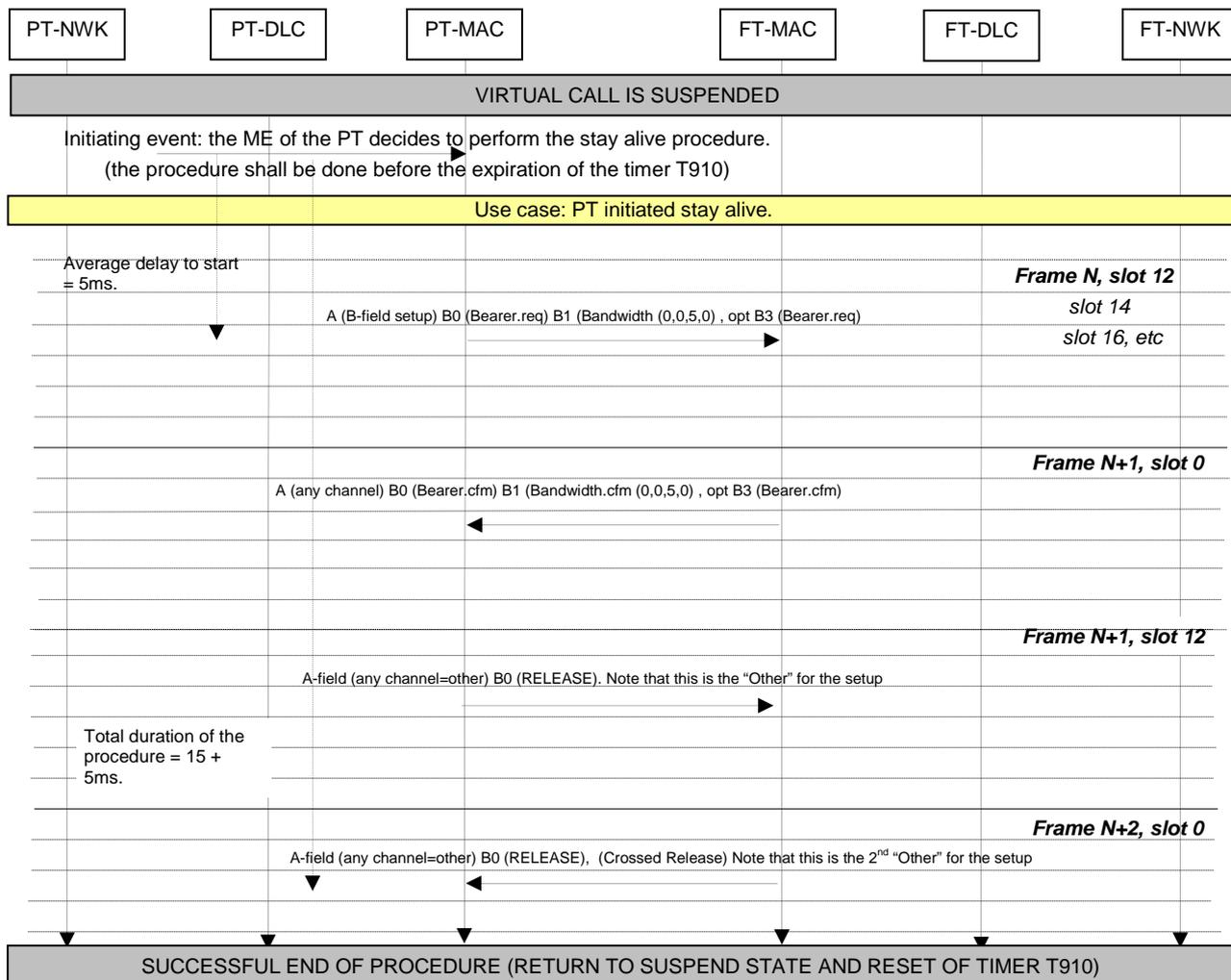
Figure E.21: Time diagram 3: optimal sequence for PT initiated stay alive procedure
