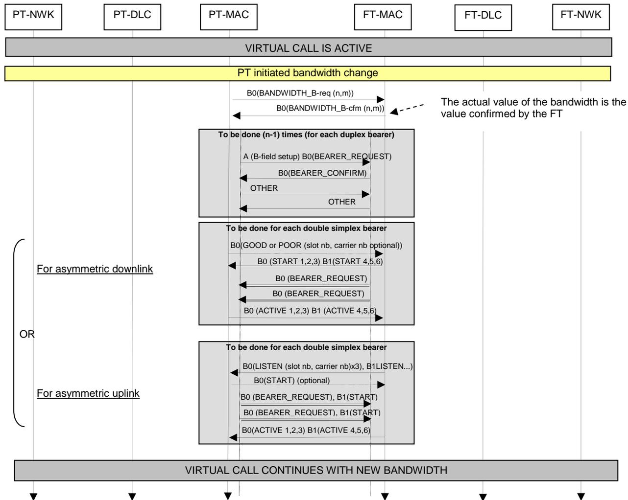
Figure E.7: Bandwidth change of the virtual call: PT initiated use case (increasing bandwidth)
