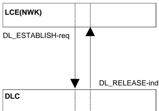
**Figure 27: Direct FT initiated link establishment failure**
