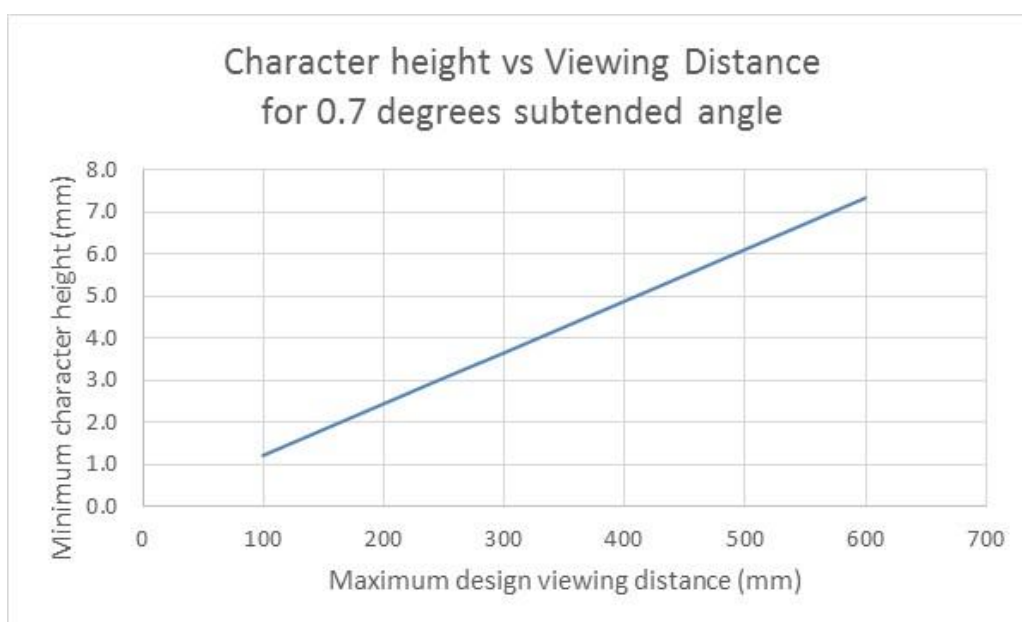
Figure 1: Relationship between minimum character height and maximum design viewing distance
