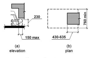
Figure 6: Toe clearance
