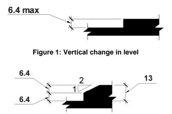
Figure 2: Bevelled change in level
