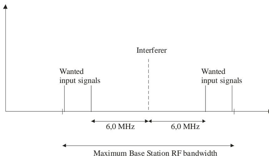
**Figure 5.3.14-1: Allocation of wanted signals and interferer**
