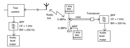
NOTE: The EUT is in position during calibration of the uplink, but not during calibration of the downlink where the EUT is replaced by the 1 kHz test audio source. During calibration of the uplink, the mouthpiece shall be placed with respect to the MRP in a way representing intended use.
