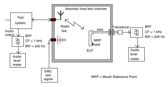
Figure B.2: Audio breakthrough measurement, test set-up for portable equipment
