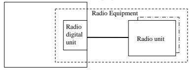
Figure 1B: BS with multiple enclosure solution
