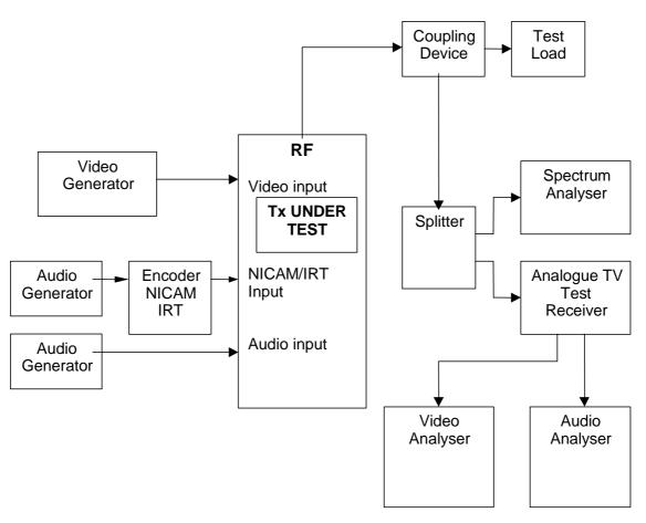
Figure 1: Typical test arrangement for the performance assessment of a standard analogue modulated TV transmitter, example
