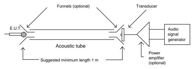
Figure 3: Example of acoustic coupling jig
