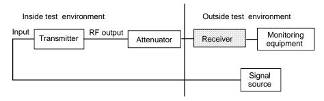
Figure 3: Test configuration for transmitters
