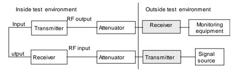
Figure 5: Test configuration of transceivers
