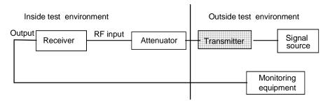
Figure 4: Test configuration for receivers
