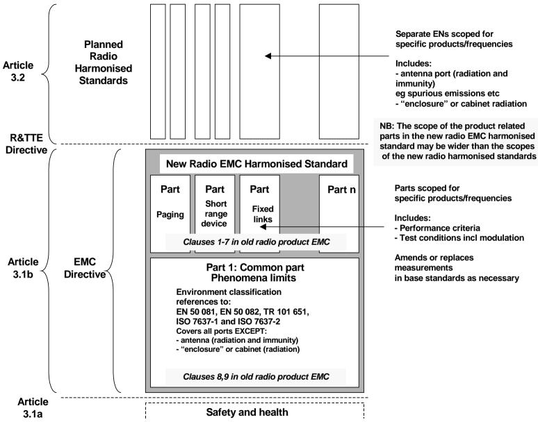
Figure 2: The new radio EMC harmonised standard
