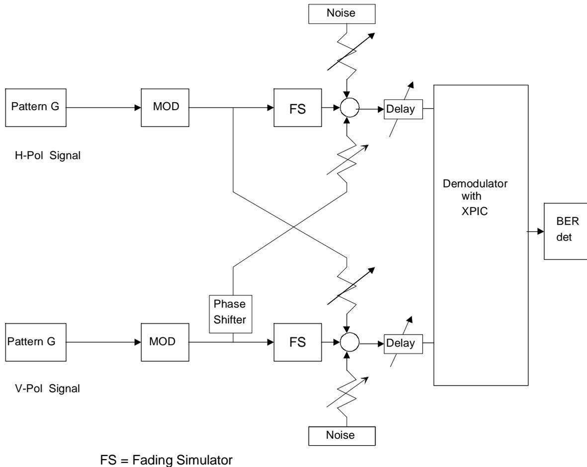
Figure A.4: Measurement test set
