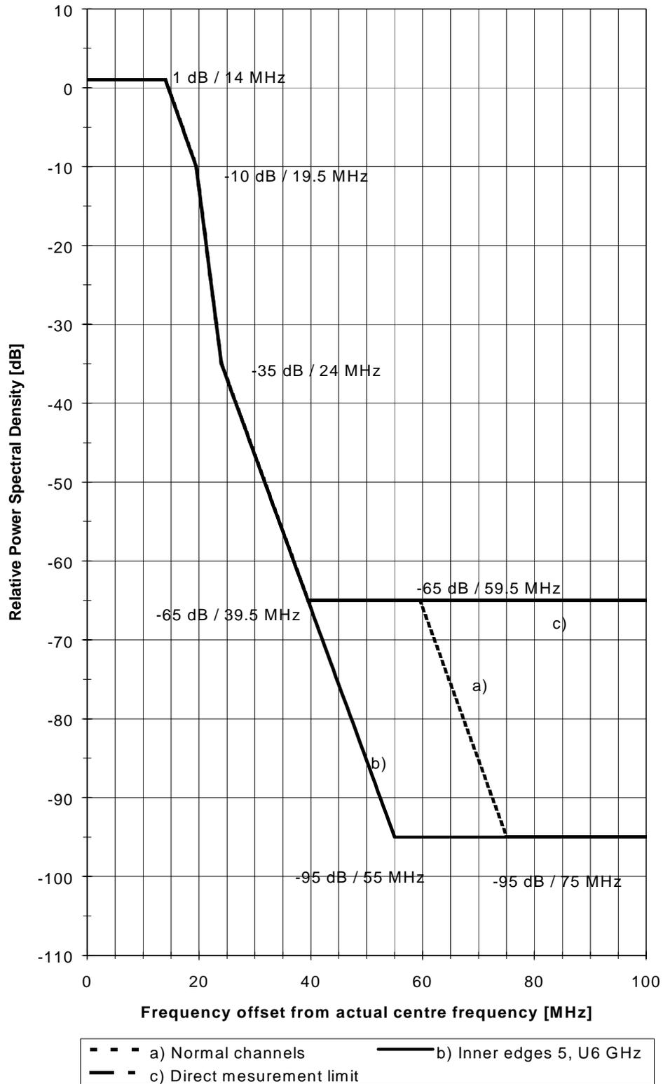
Figure 3: Limits of power spectral density
