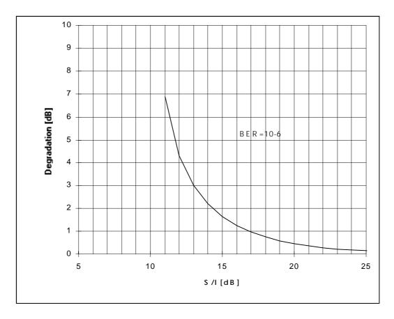
Figure A.3: Co-channel (internal) interference threshold degradation referenced at point B (or C)
