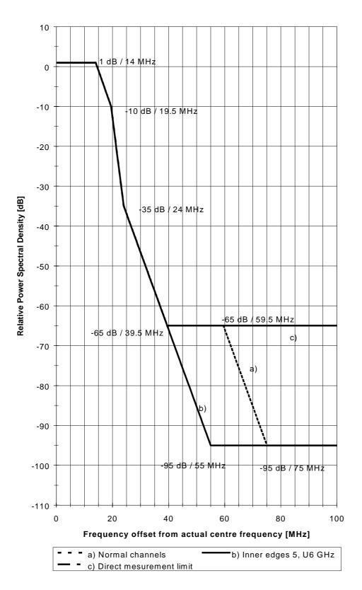
Figure 2: Limits of power spectral density
