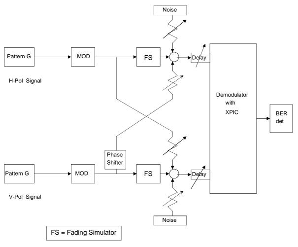
Figure A.4: Measurement test set
