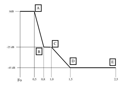
Figure 1: DS-CDMA spectrum mask normalized for channel spacing
