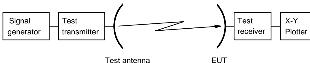
Figure 12: Test arrangement - transmit polarization discrimination
