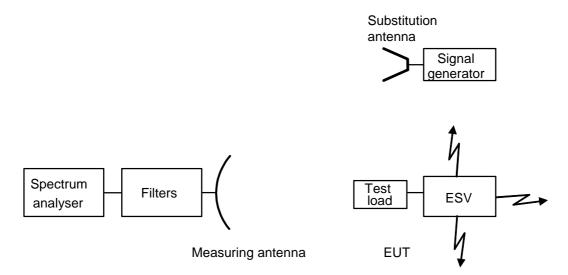
Figure 4: Recommended test arrangement-spurious radiation measurements above 2 000 MHz for an EUT without antenna
