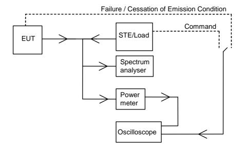
Figure 13: General test arrangement for control and monitoring tests for conducted measurements
