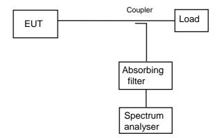
Figure 6: Test arrangement - on-axis spurious radiation measurements at the antenna flange
