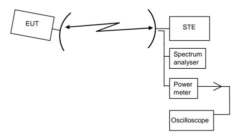
Figure 11: Test arrangement for pointing error detection
