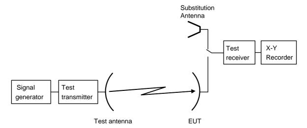
Figure 9: Test arrangement-antenna transmit gain measurement
