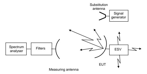
Figure 3: Test arrangement-Spurious radiation measurement above 2 000 MHz for an EUT with antenna
