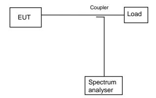
Figure 8: Test arrangement-transmit output power density measurement
