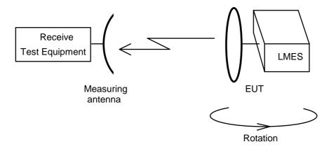
Figure 2: Test arrangement - emissions measurement, first axis
