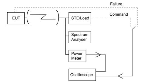
Figure 5: General test arrangement for control and monitoring tests for radiated measurements
