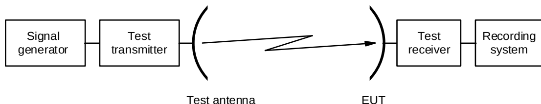
Figure 11: Test set up - antenna transmit radiation pattern measurement
