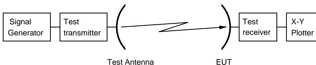
Figure 11: Test arrangement - antenna transmit radiation pattern measurement
