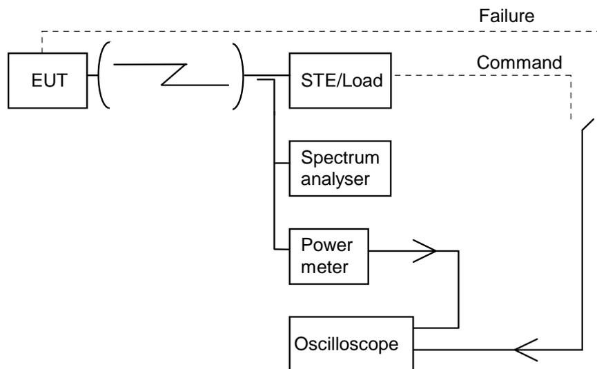
**Figure 14: General test arrangement for control and monitoring tests for radiated measurements**
