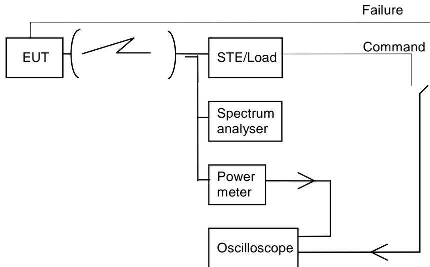
**Figure 13: General test arrangement for control and monitoring tests for radiated measurements**
