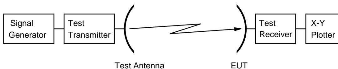
**Figure 16: Test arrangement - antenna receive pattern measurement**
