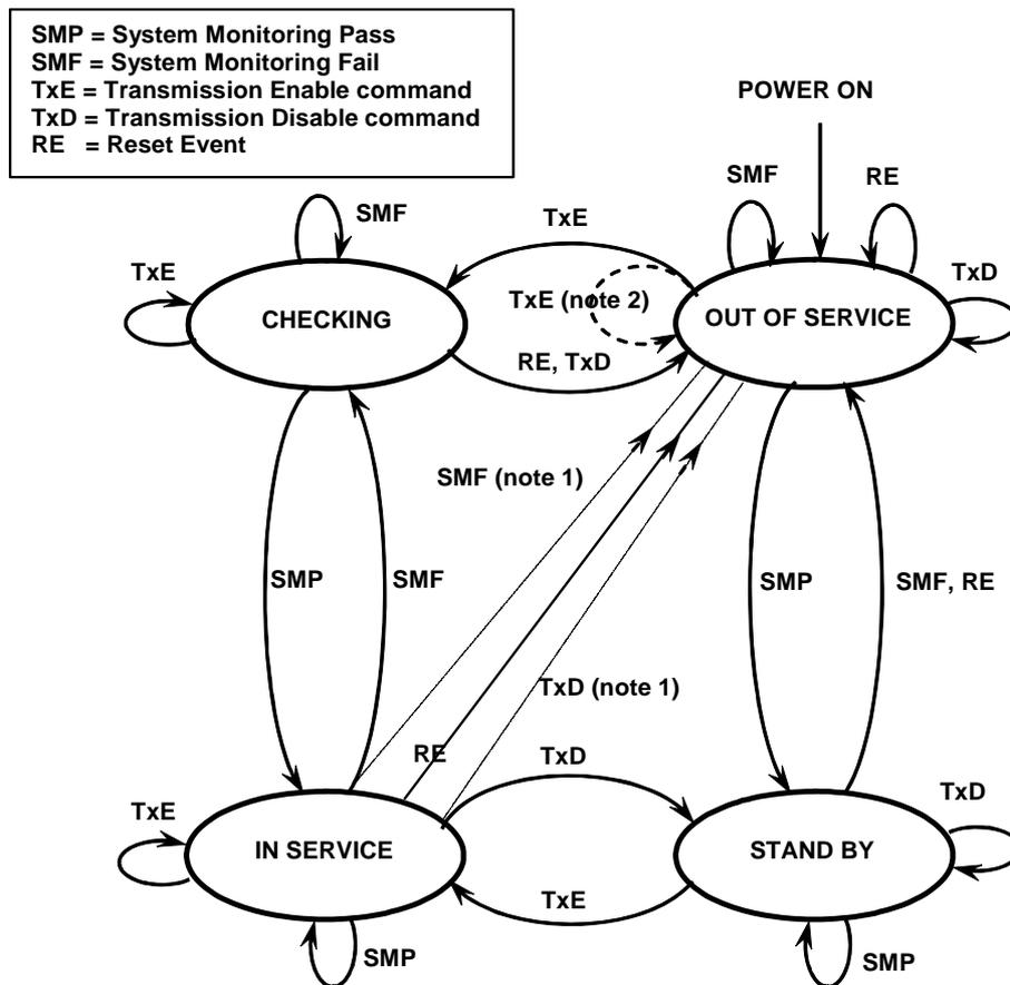
NOTE 1: In the "in-service" state, the occurrence of a SMF and/or TxD may result in a transition to the "out-of-service" state.
