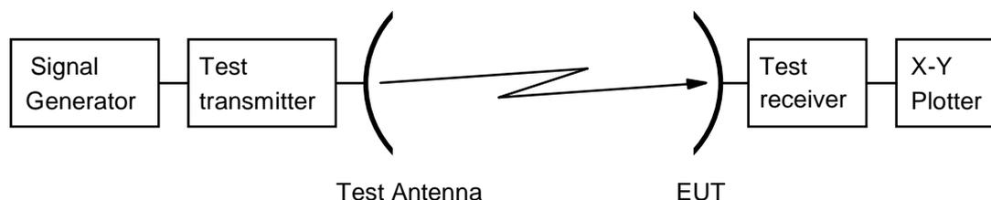
**Figure 11: Test arrangement-antenna transmit radiation pattern measurement**
