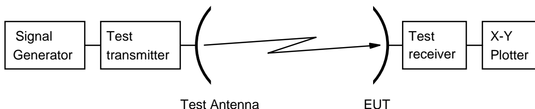
Figure 11: Test arrangement-antenna transmit radiation pattern measurement
