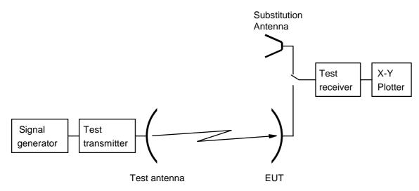
Figure 10: Test arrangement-antenna transmit gain measurement
