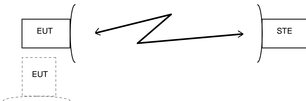
Figure 10: Test arrangement - static rms pointing accuracy
