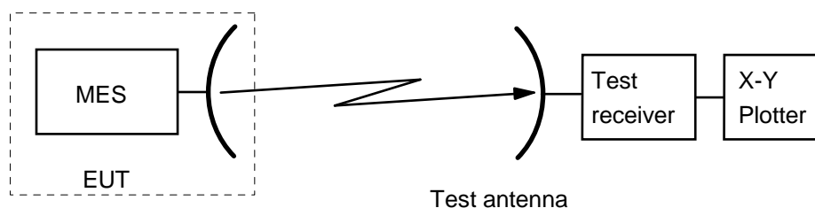
Figure 16: Test arrangement - antenna transmit radiation pattern measurement
