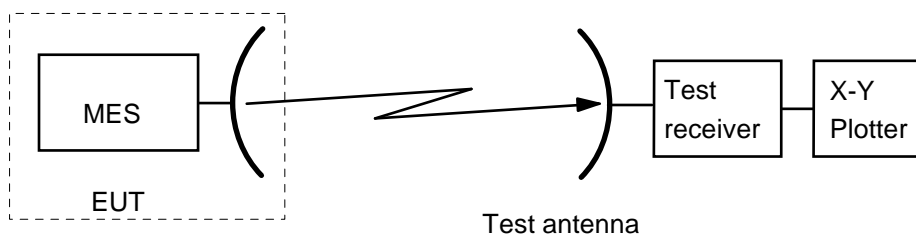
Figure 16: Test arrangement - antenna transmit radiation pattern measurement
