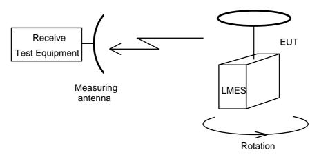
Figure 4: Test arrangement - Unwanted emissions measurement, third axis
