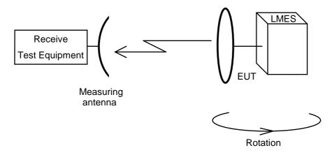
Figure 3: Test arrangement - Unwanted emissions measurement, second axis
