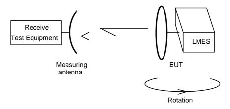
Figure 2: Test arrangement - Unwanted emissions measurement, first axis
