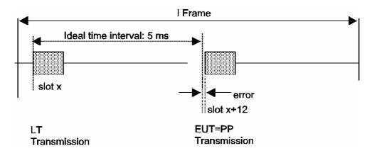
Figure 33: PP packet transmission error definition
