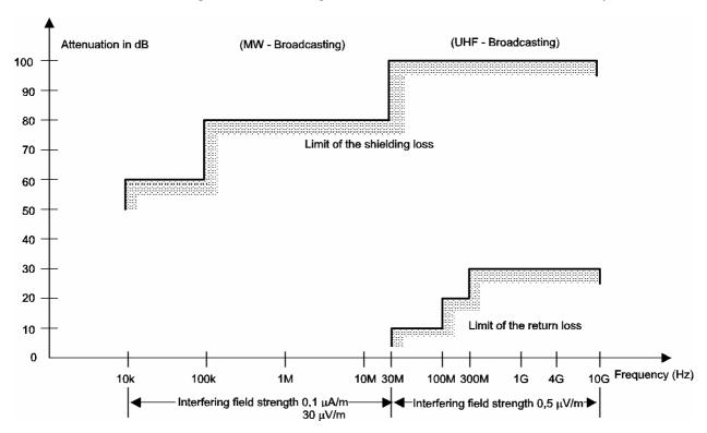
Figure 12: Shielding and wall return loss
