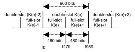
Figure 4: Double-slot format
