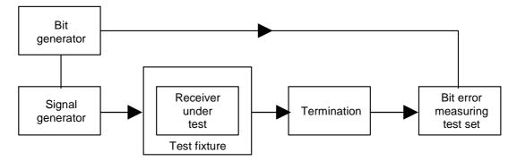
Figure B.2: Measurement arrangement No.2
