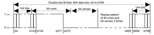
NOTE: Bits  $b_0$  to  $b_{143}$  and  $b_{656}$  to  $b_{799}$  are alternating 1s and 0s.
