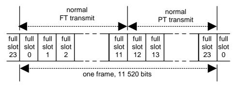
Figure 2: Frame and full-slot structure
