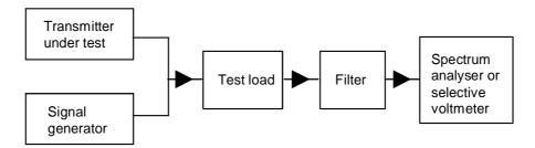
Figure C.1: Test set up
