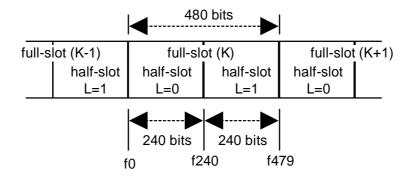
Figure 3: Half-slot format
