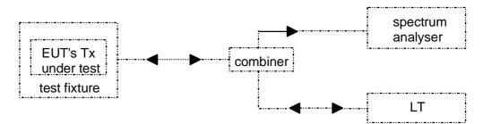
Figure 14: Measuring arrangement for calibration
