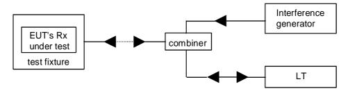
Figure 15: Measuring arrangement for calibration
