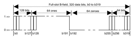
NOTE: Bits  $b_0$  to  $b_{127}$  and  $b_{256}$  to  $b_{319}$  are alternating 1s and 0s.
