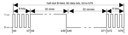
NOTE: Bits  $b_0$  to  $b_7$  and  $b_{72}$  to  $b_{79}$  are alternating 1s and 0s with the even order bits ( $b_0$ ,  $b_2$ ,  $b_4$ ,...) set to "1" and the odd-order bits ( $b_1$ ,  $b_3$ ,  $b_5$ ,..) set to "0".
