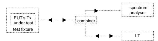
Figure 14: Measuring arrangement for calibration
