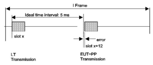
Figure 33: PP packet transmission error definition
