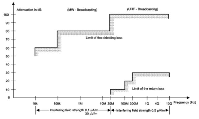
Figure 12: Shielding and wall return loss
