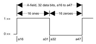
Figure 35: Test packet structure for case 2, A-field
