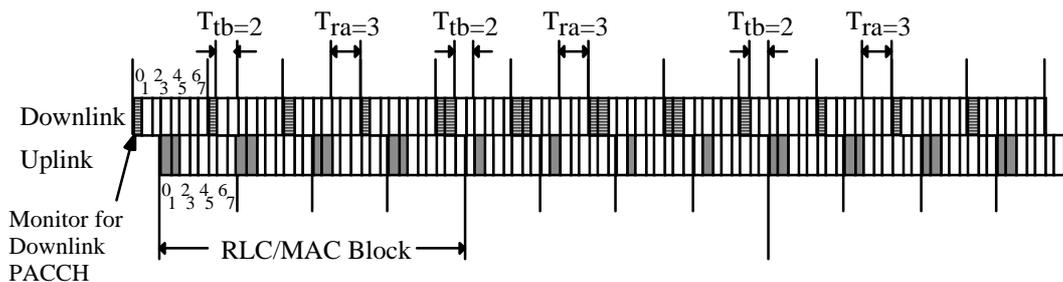
**Figure D.6: Multislot Class 3 (Rx=2, Tx=2,Sum=3), 2 timeslot uplink TBF, the first uplink timeslot in the second block is not allocated in the Allocation Bitmap**
