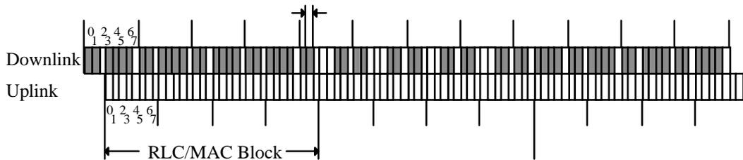
**Figure D.16: Multislot Class 21 (Rx=6, Tx=4, Sum=NA), 6 timeslot downlink TBF, no uplink TBF, with a 2 timeslot Measurement Mapping block**
