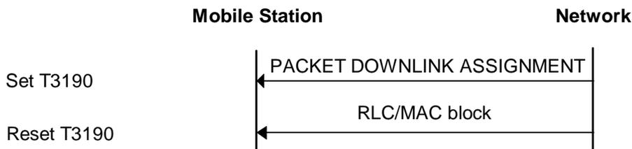
Figure C.2: TBF establishment initiated by the network
