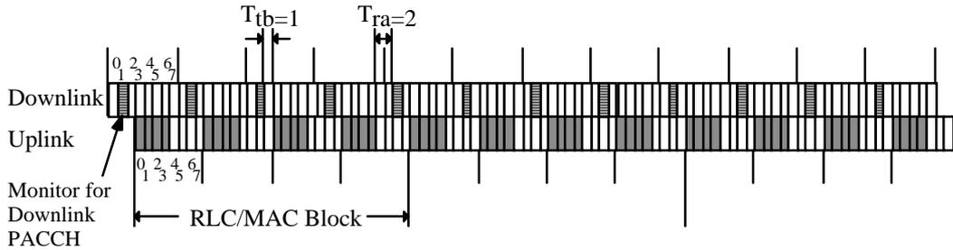
**Figure D.12: Multislot Class 21 (Rx=6, Tx=4, Sum=NA), 4 timeslot uplink TBF**
