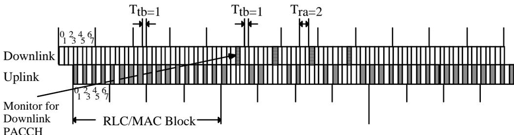
**Figure D.14: Multislot Class 21 (Rx=6, Tx=4, Sum=NA), 4 timeslot uplink TBF, with a PACCH opportunity due to a gap in Fixed Allocation**
