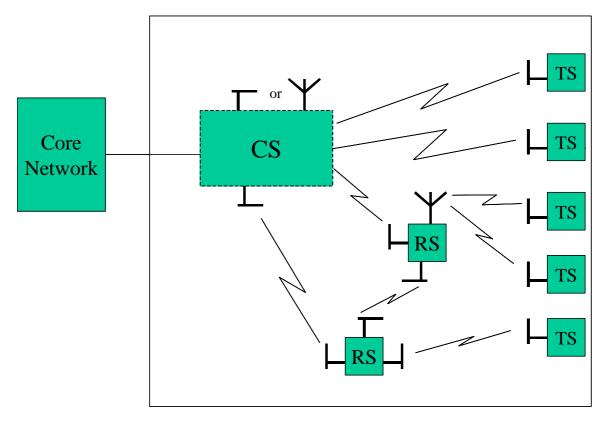
**CS**: Central Station, which is linked to remote stations (repeater or terminal stations) by microwave transmission paths.
