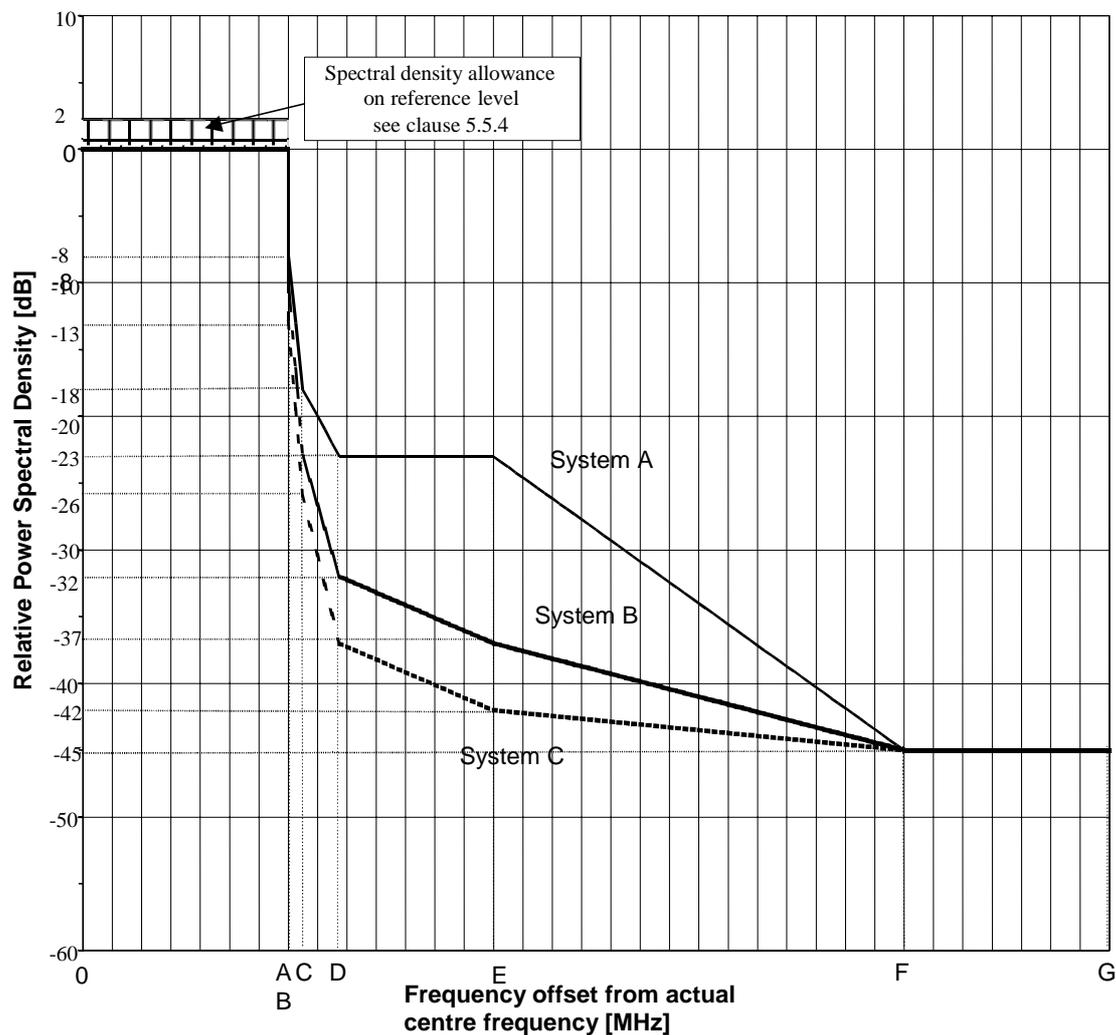
Figure 2: Spectrum masks of the composite multi-carrier system ( $f_0$  = channel centre frequency)
