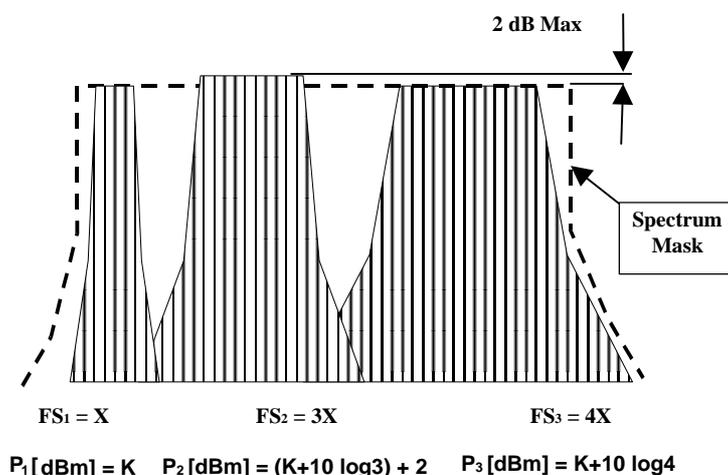
**Figure 1: Example of three sub-carrier system with different symbol frequency (FS)**
