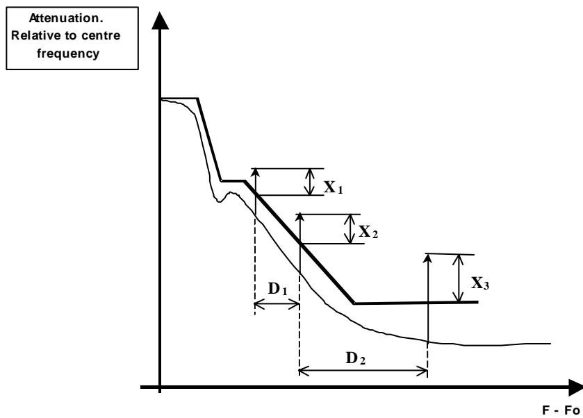
**Figure 2: CW lines exceeding the spectrum mask (typical example)**
