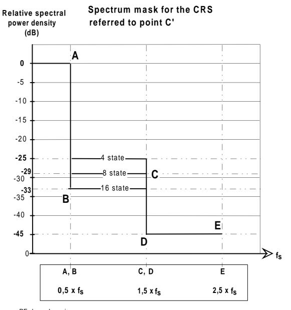
f<sub>s</sub>: RF channel spacing NOTE: The different spectral power
